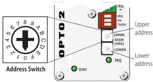
Each B3000-B contains four addresses: the base address, base +1, base +2, and base +3. The base address is an even multiple of 4.
