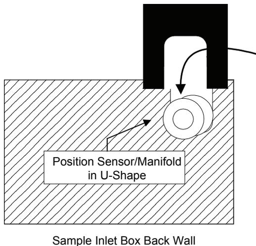
3. Set the turbo pump between the guides and rotate until you have positioned the sensor/manifold correctly in the U-shaped slot on the sample inlet wall. Once it is in the correct position, slide the clip onto the pump to lock it into position.
