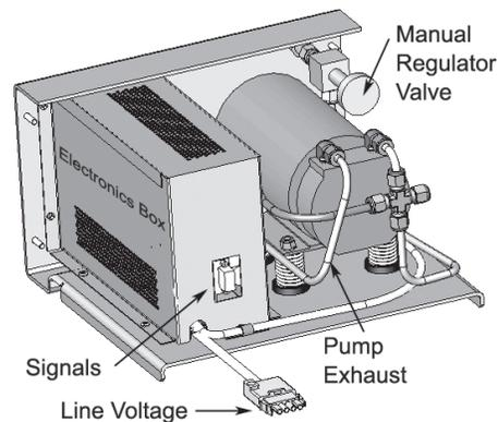
7. Attach the power cable (white connector) on the extended pressure range module to one of the three line voltage outlets on power distribution box on the underside of the ProLine (Figure A2-5).
