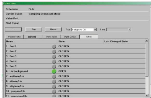
to change the valve from closed to open (green). All valves should have a green indicator showing they are all open.
